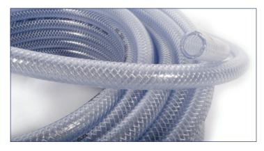
An economical, light duty hose ideal for multi-purpose use, PVK Glass Clear is especially popular for industrial airline equipment. It can also be used for food contact applications. Manufactured from transparent, low toxic PVC and reinforced with high tensile polyester fibres.
