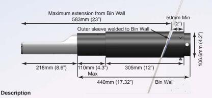
Hydro-Probe II - Standard Mode for normal digital or analogue connection
