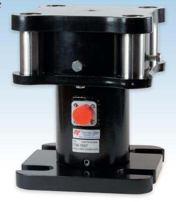
A stainless steel compression load cell housed in an integral mounting assembly, which is ideal for general commercial weighing of large tanks, silos and vessels, particularly in the cement, minerals and coal industries. The design ensures optimum performance and eliminates many traditional problems encountered during the installation of high capacity weighing systems. The T30 load cell and mounting assembly are supplied as a complete locked unit, ready to install.
