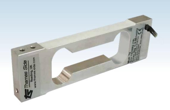
This double bending beam single point load cell is manufactured from high quality aluminium alloy. Its design allows for high accuracy weight measurement with off-centre loads. It's potted and sealed to IP66.
