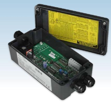
The XTSGA Load Cell Amplifier is a versatile signal conditioning unit for silo weighing, process control and PLC interface applications. It can be powered from 110/230 VAC or 18-24 VDC (selected at time of order) and provides very stable excitation for up to 4 x 350 ohm load cells. It is housed in a black surface mounted ABS case, with IP65 environmental protection and full CE compliance. An optional isolated power supply module can extend the DC power range from 9 to 36 V.
